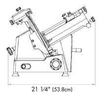
Controls: Manual slice thickness knob, push button on/off, attached blade sharpener
