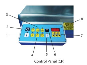
To turn the blade off, press the blade off button (CP [2]).
