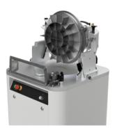
**4.** Press the "Start" button "a"; the knives will exit the machine for cleaning
