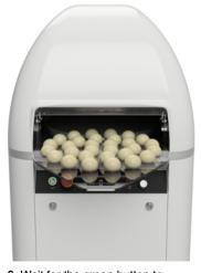
Wait for the green button to flash;Open the guard casing and remove the plate with shaped balls
