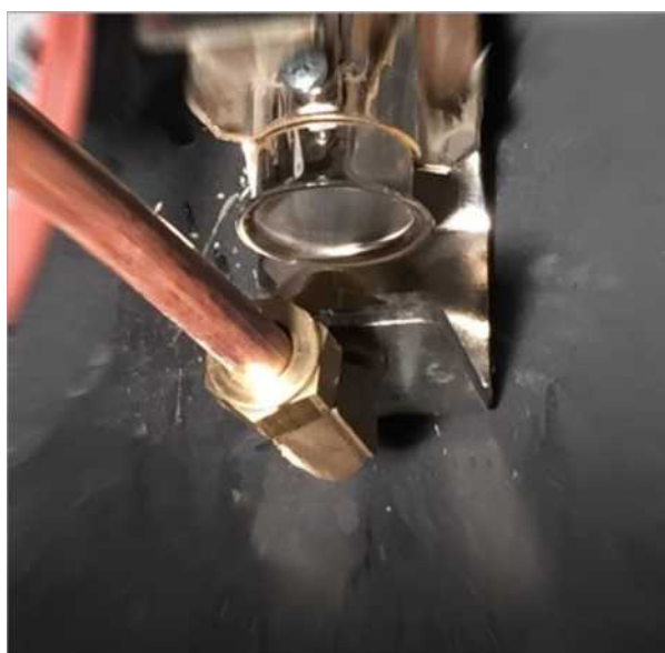
Fig 7.2 Nozzle-holder curve and damper sleeve
