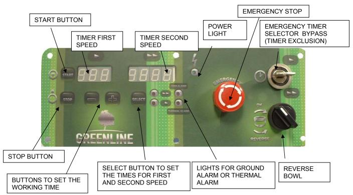
The control panel is used for the operation of the spiral mixer by the user. In order to operate the control panel, the Mains Power Switch (left side of the machine) must be switched on.
