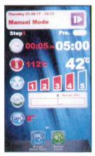
After starting the programs the parameters Time, Temperature, Fan speed, Climate, Steam injection, keep on being modifiable for the running program. Touch the corresponding icon to access the modification of the parameter.
