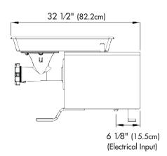
**Motor:** 1 hp grease packed gear motor provides compact, smooth, and quiet performance with an 8:1 reduction within the gear motor resulting in a 224RPM drive shaft output. Worm is coupled directly with the gear output shaft.
