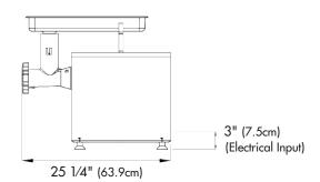
Motor: 1 hp capacitor start, 1740RPM, ball bearing motor mounted on cushioned supports for noise and vibration reduction.
