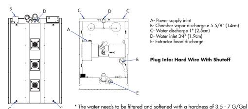
A- Power supply inlet B- Chamber vapor discharge ø 5 5/8" (14cm) C- Water discharge 1" (2.5cm) D- Water inlet 3/4" (1.9cm)
