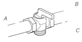
A. To range B. Manual shutoff valve "closed" position C. Gas supply line
