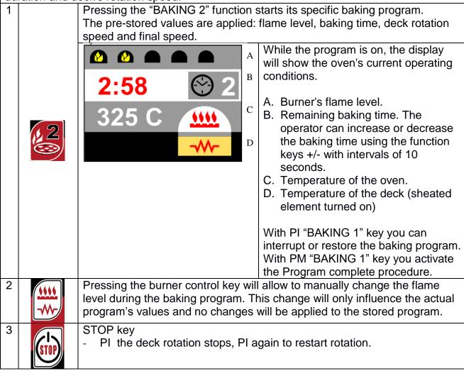
The operating modes of the "BAKING 1" function keys are totally similar to the "BAKING 2" key modes.
