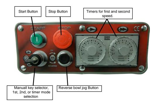
The control panel is used for the operation of the spiral mixer by the user. In order to operate the control panel, the Mains Power Switch (left side of the machine) must be switched on.
