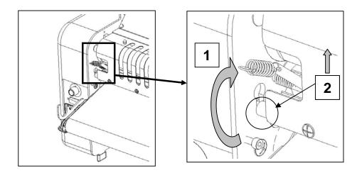
Press the spring at the left end of the scraper (3) and extract the opposite end. Do the same for the scraper inside
